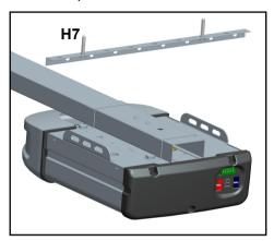
**5.5** Cut the hanging brackets to measured lengths.
