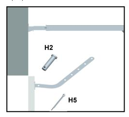
7.2 Pull the emergency release to move the trolley to the locking holes. Connect the straight door arm to the trolley by using the shouldered shaft (H2). Attach the shouldered shaft with the cotter pin.
