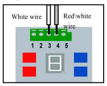
**Note:** To connect or disconnect the wires from the terminal, press in the tab with a screwdriver tip.
