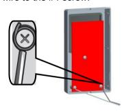
10.5 Insert and tighten screws to secure the back cover of the wall control to wall.
