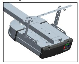
**5.7** Fasten the hanging bracket on the chassis of garage door operator with bolts (H4),and nuts (H3).
