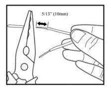
11.2 Connect the white wire to the #3 terminal and the red\white wire to the #4 terminal on garage door operator.
