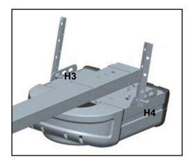
**5.8** Open and close the door manually. If the door hits the rail, lift the header bracket.
