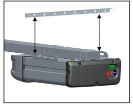
**5.6** Fasten the end of each hanging bracket to the bracket on the ceiling.
