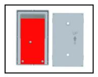
**10.4** Mark the location of the 2 holes of back cover of wall control and drill a 6 mm hole.
