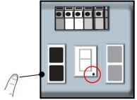
**6.2** Within 10 seconds, press the **Button 1** on the remote control, the "●"will turn off. Press the **Button 1** again, the "●" will flash and turn off. Now, congratulation!
