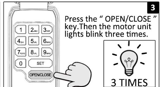
According to the above steps, the master password sets successfully. (\*One key to open and close until the door is fully closed\*)
