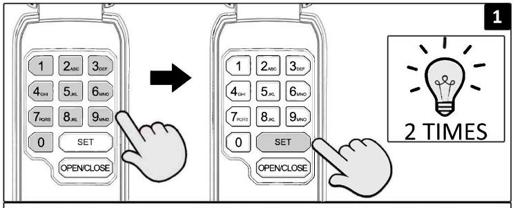
Enter the master password, hold the "SET" key. Then the motor unit lights blink twice.
