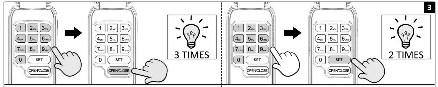
Enter *number of hours*(1~255) for temp PIN to last and hold the "OPEN/CLOSE" key until motor unit lights blink three times.
