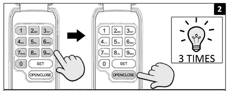
Enter new three to six digit temporary PIN. Hold the "OPEN/CLOSE" key until motor unit lights blink three times.
